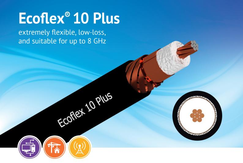
Ecoflex 10 Plus is a highly flexible, low-loss coaxial cable specifically designed for operation up to 8 GHz. State-of-the-art production methods and the use of a low attenuation PE-LLC dielectric with a gas content of over 70% enable very low attenuation values. The Ecoflex 10 Plus sets new standards for flexible coaxial cables.
